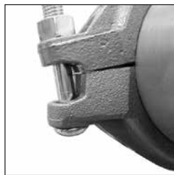
Excess Torque or Shallow Groove Dimension
