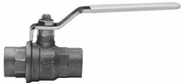
Lead Free* Brass Ball Valve – Solder 1615 LF 1/2" - 3" Full Port Connection: ANSI B 16.18 - Solder Ends
