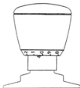
Figure 3 - With no arrows visible, the Inner Scale set at 4 and the indicator line aligned with the Outer Scale 0; the valve setting is 4.0 and the valve is fully open.
