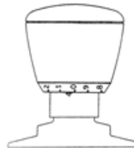
Figure 3 – With no arrows visible, the Inner Scale set at 4 and the indicator line aligned with Outer Scale 0; the valve setting is 4.0 and the valve is fully open.
