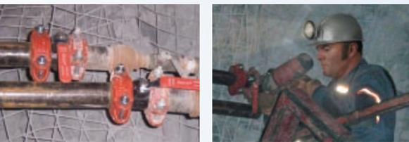
*Pictured left to right at top are Western Nevada Supply owners Rick, Jack, and Ted Reviglio. Pictured to the lower left is Grovlok couplings and valves installed along the upper wall of a hard rock mine shaft. Pictured to the lower right is a miner actually installing a Grovlok 7001 coupling with one bolt to complete the assembly – fast and easy.*
